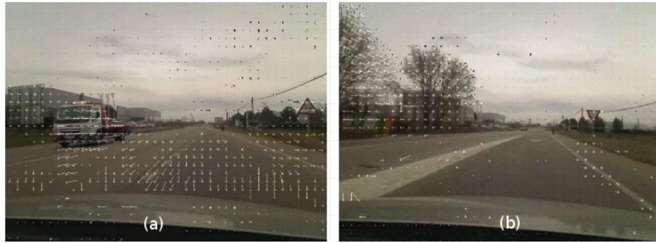
Fig. 2. Comparison of vectors in a frame with an object and another with no one
